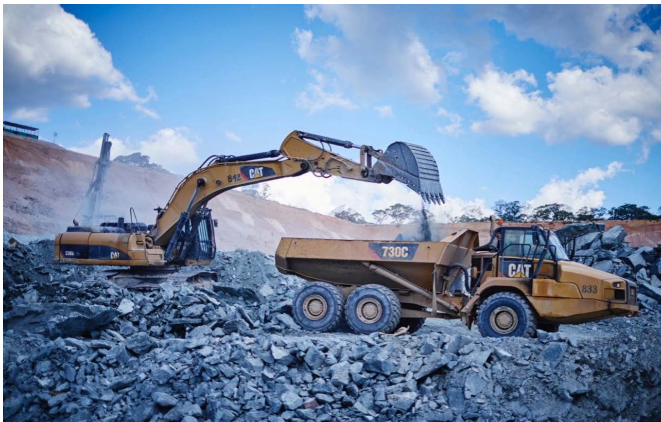
Removing bedrock at an open-pit mine using heavy machinery to reach the gemstone-bearing rocks. (Photo courtesy of Gemfields.)
